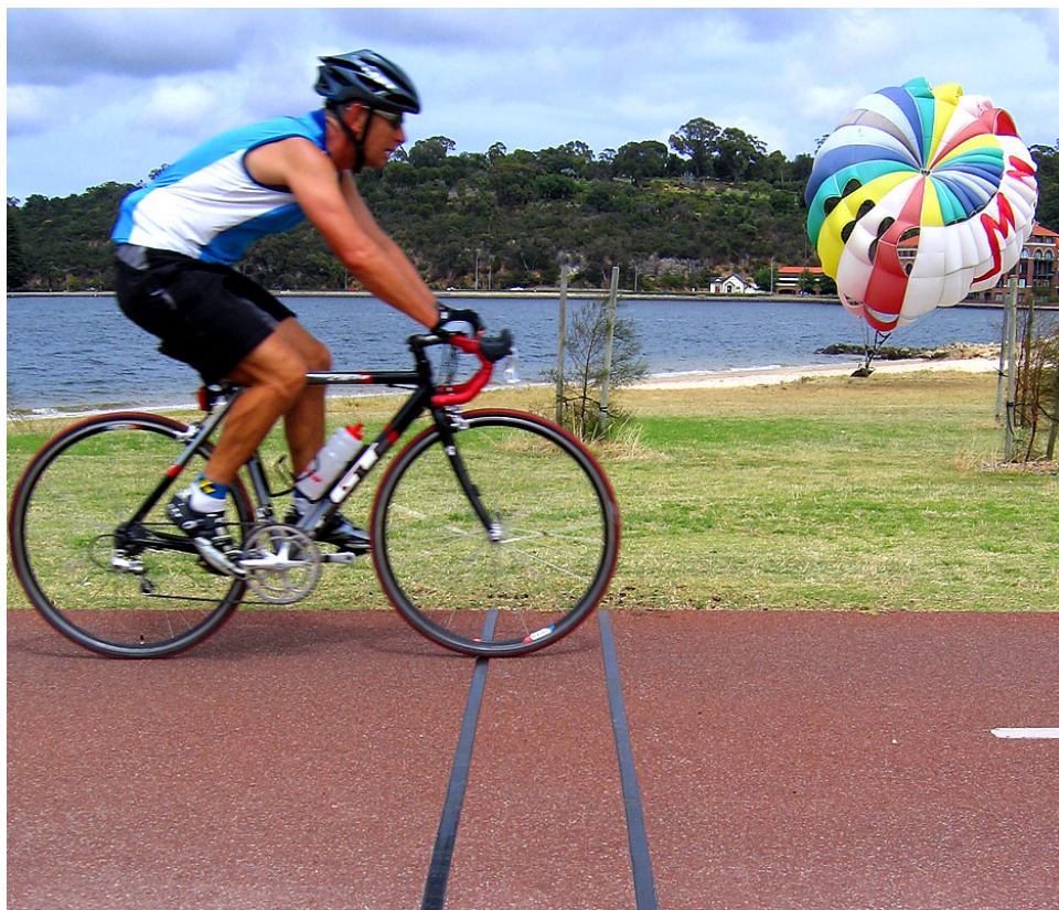
Embedded piezo sensors for the MetroCount 5720
