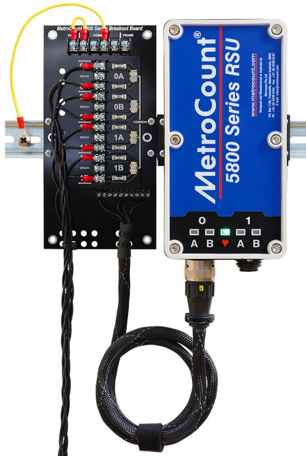
MC5810 Loop Classifier with Breakout Board
